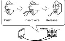
Once your AV receiver is ready for use, you'll need to tune into an AM radio station and adjust the position of the AM antenna to achieve the best possible reception.
